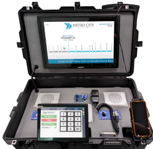
Bus in box - Portable training aid for on-board bus technologies
