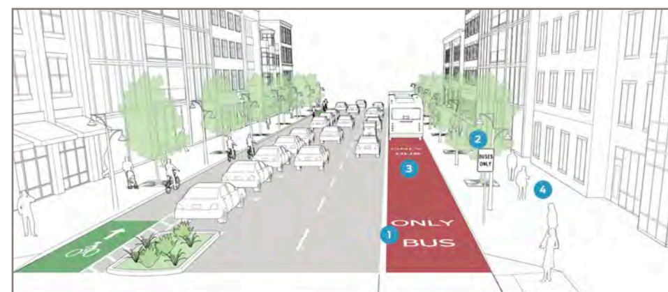
Figure 61: Bus Lanes and Transit Signal Priority can prevent declines in speed and reliability as Missoula grows. (Illustration from NACTO Transit Street Design Guide.)
