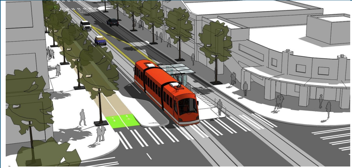
Seattle's First Hill Streetcar line (under construction) includes a protected two-way cycle track parallel to the streetcar/traffic lanes.
